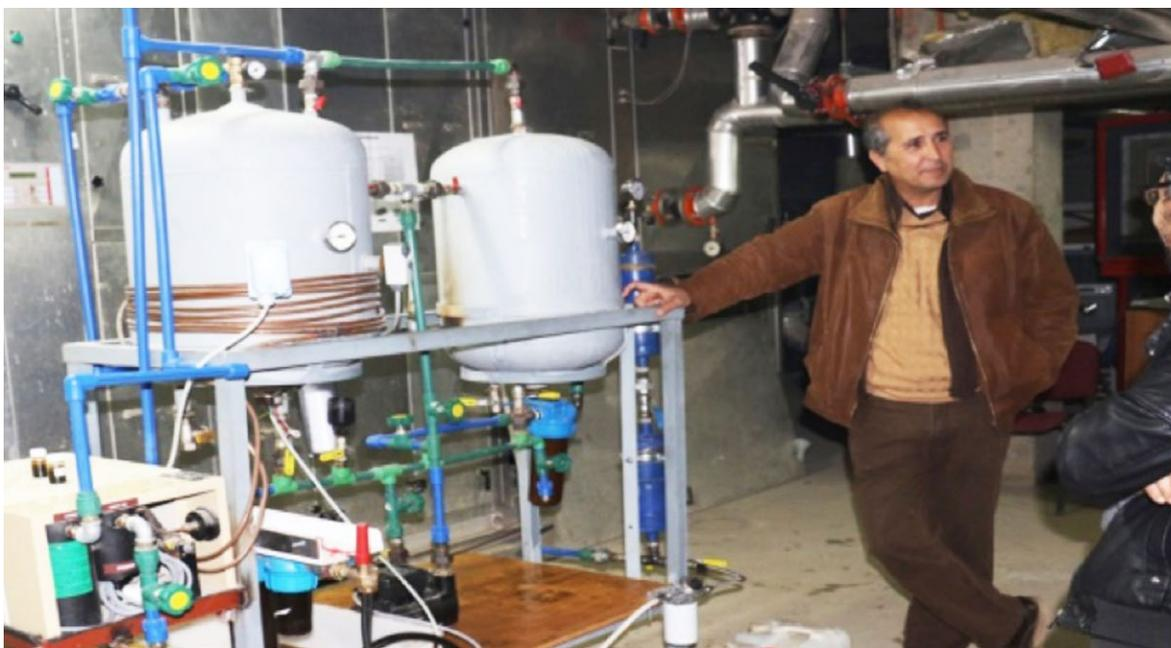
A project funded by an AUI Seed Money Grant has developed a small-scale converter which processes used cooking oil into biodiesel fuel. In contrast to large, expensive systems, this converter uses mostly recycled materials. Tests show that it produces cleaner fuel and also allows the users to collect byproducts such as glycerin which can be used for other purposes.
